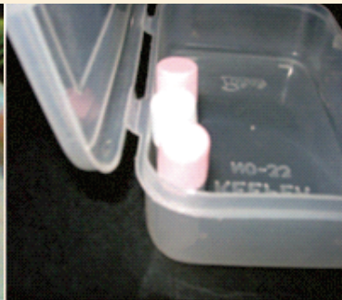
Fig 36: Sample transportation box or tiffin box for school kids. Use appropriate sample transportation box with numbered lid to avoid leakage of specimens during transport.
